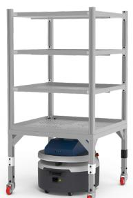
Fetch100 Connect Automatically pick up and drop off carts up to 125 lbs. (57 kg)
