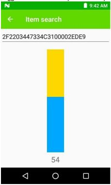
5. Tap on Relative distance to see varying relative distance of tags in field of view based on their RSSI as detected by reader. It is based on color heat map where blue (cold) to red (hot) for far to near tag respectively.
