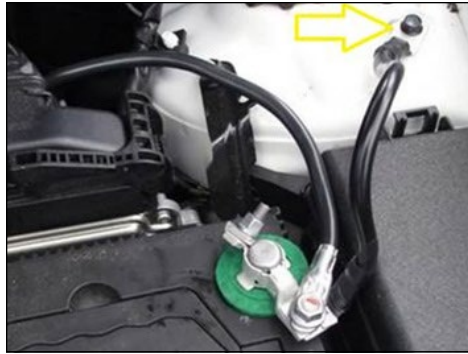
Figure 4: Heavy Wire Connecting to Chassis
