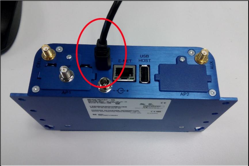
Figure 8 – Plugging in the USB cable
