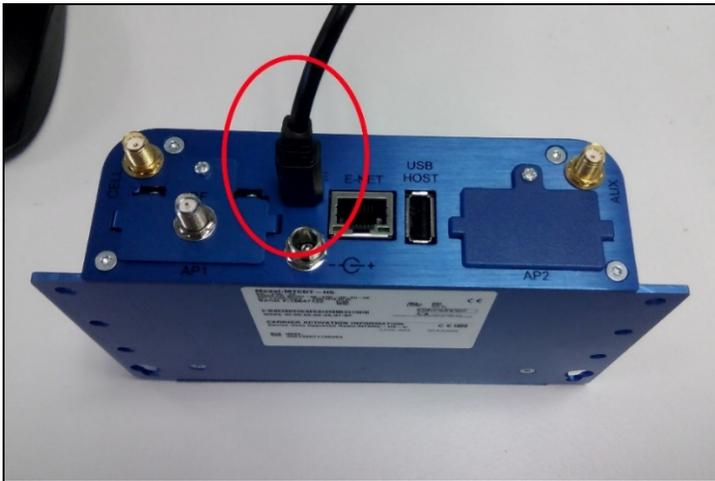
Figure 4 – Plugging the USB cable
