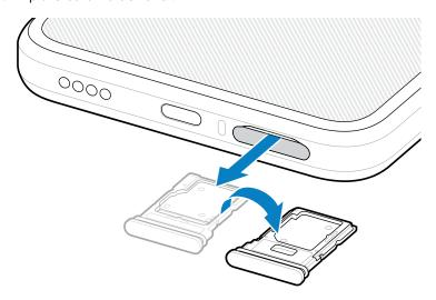
**3.** Place the SIM card end, with contacts facing up, into the card holder.
