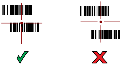
Figure 7 RS5100 Pick List Mode with Multiple Barcodes in Aiming Pattern
