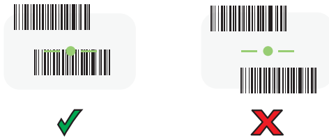
Figure 10 RS6000 Pick List Mode with Multiple Barcodes in Aiming Pattern
