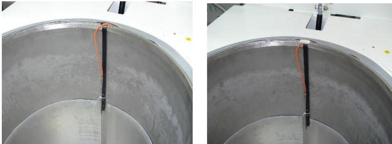
*Figure 8 – PT100 (-200°C to +50°C) for nitrogen/cryogenic tank*
