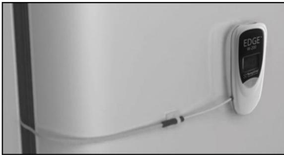
*Figure 12 – EDGE module mounted on the refrigerator door*
