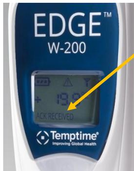
Figure 4 – Confirming connection with LoRa Gateway receiver
