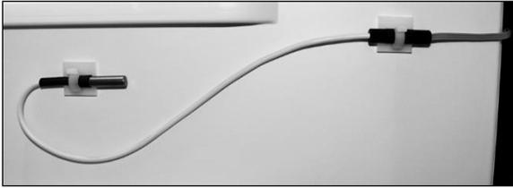
*Figure 11 – Sensor inside refrigerator chamber (modules with external sensor only)*
