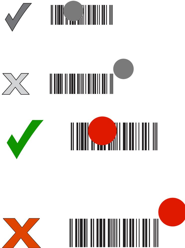
The aiming dot is smaller when the scanner is closer to the barcode and larger when it is farther away. Scan barcodes with smaller bars or elements (mil size) closer to the scanner and those with larger bars or elements (mil size) farther from the scanner.
