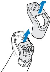
3. Insert/remove the battery.
