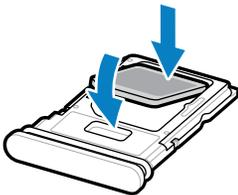
4. Press the SIM card down into the card holder and ensure that it seats properly.
