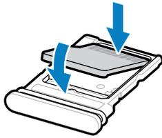
3. Press the card down into the card holder and ensure that it seats properly.
