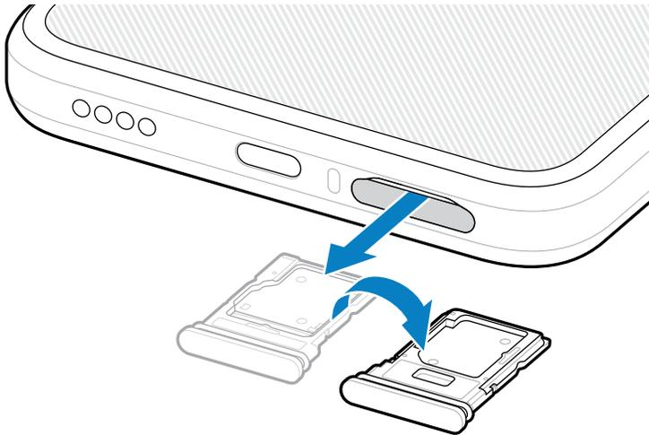
3. Place the SIM card end, with contacts facing up, into the card holder.
