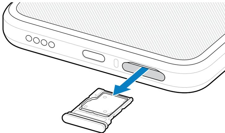
2. Place the microSD card, contact end first, with contacts facing up, into the card holder.
