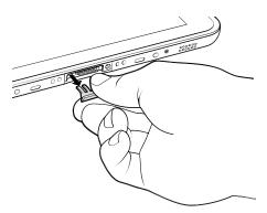
3. Insert the Rugged IO Adapter (2) onto the tablet interface connector (1).
