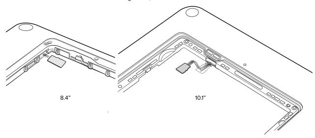
**2.** Push the micro SD card in and ensure that it locks into place.
