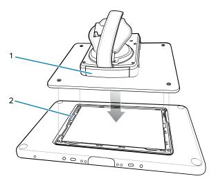
**5.** Using a T6 Torx screwdriver, secure expansion back to device using four screws (1). Torque to 14 n-cm.
