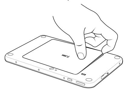
**4.** Carefully lift the battery cover off the device.
