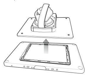
**4.** On 8 in. version only, replace rubber gasket removed during installation.
