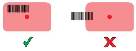
**6.** Upon successful decode, the scanner beeps and the LED flashes, and the scan line turns off. The captured data appears in the text field.
