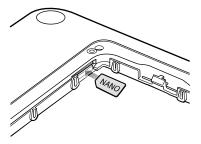
Figure 7 Inserting the nano SIM Card - 10 in.
