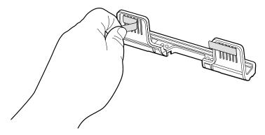
2. Align the tall insert over the pins.
