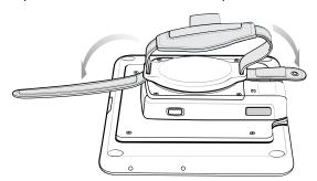
**4.** Pull the strap end without the eyelet through the slot on the Expansion Back.
