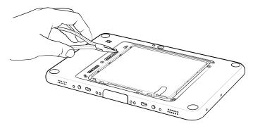
**4.** Align expansion back with device. Ensure that the power pack slot cover (1) is aligned with the bottom of the device and the interface connector (2) on expansion back aligns with interface connector on device.
