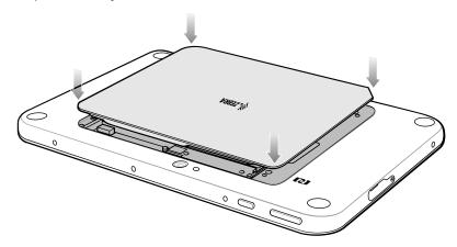
**6.** Carefully press down around the edge of the cover. Make sure that the cover is seated properly.
