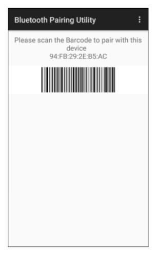
4. Using the Bluetooth scanner, scan the barcode on the screen.
