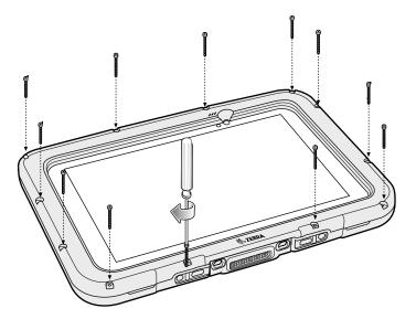
Figure 54 Secure 10 in. Rugged Frame
