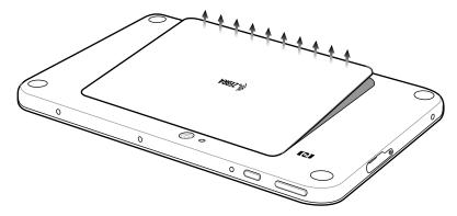
**5.** On the 8.4 inch version, push the two locking tabs (1) up, then pull up on the tab (2) to remove battery.
