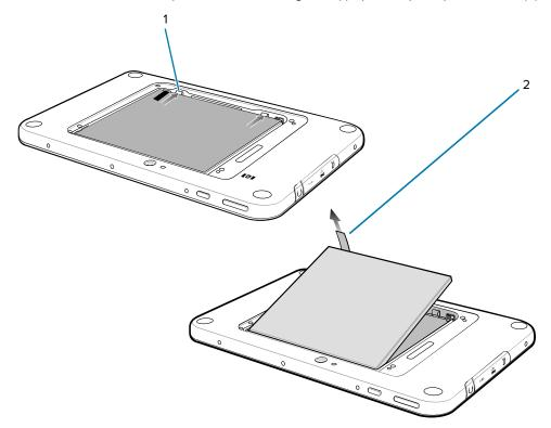
**6.** On the 10.1 inch version, push the two locking tabs up (1), then lift the battery up (2).
