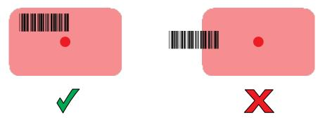
When the Integrated Scanner is in Pick List mode, the device does not decode the barcode until the aiming dot touches the barcode.
