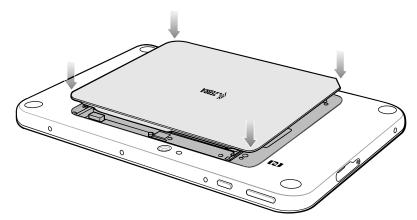
**6.** Carefully press down around the edge of the cover. Make sure that the cover is seated properly.
