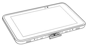
2. If installing the Rugged IO Adapter, pull the access cover away from the device until it separates from the device.
