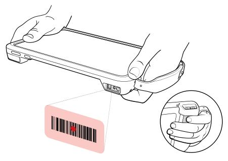
**4.** Ensure the barcode is within the area formed by the aiming pattern.
