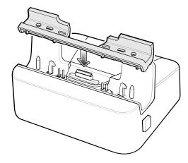
2. Press the insert down until it seats flush in the cradle.
