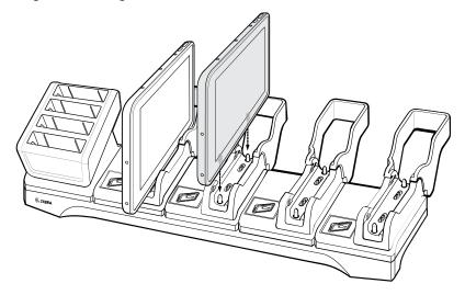
**3.** Place the device down into the slot with display facing away from Battery Charger.
