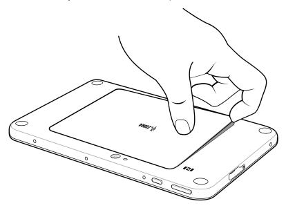
**3.** On 8.4 in. version only, remove rubber gasket.
