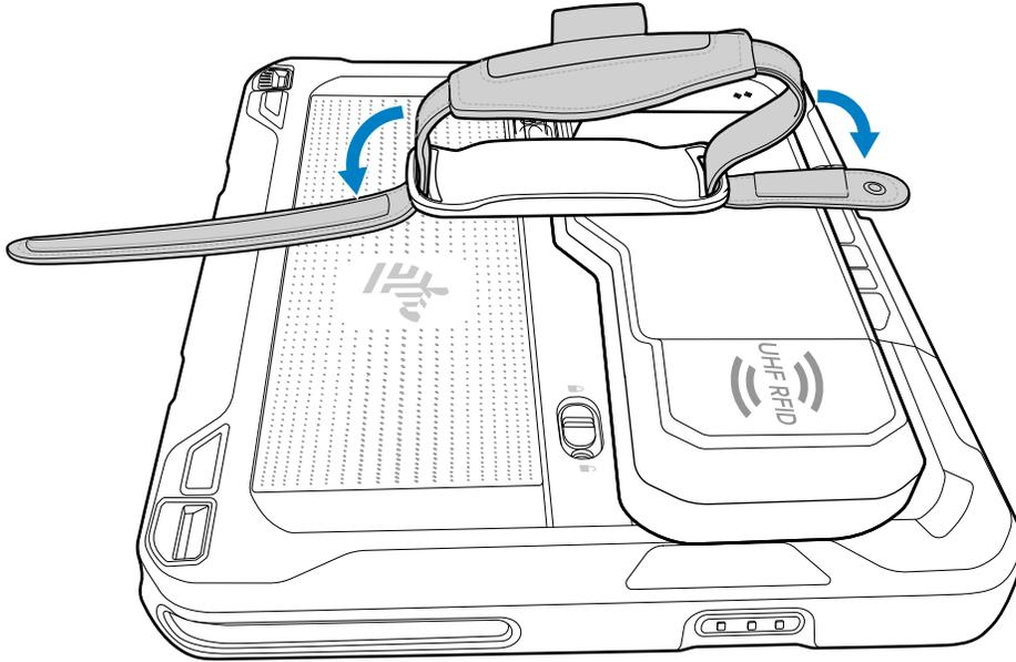
2. Pull both ends of the hand strap through the slots in the reader.
