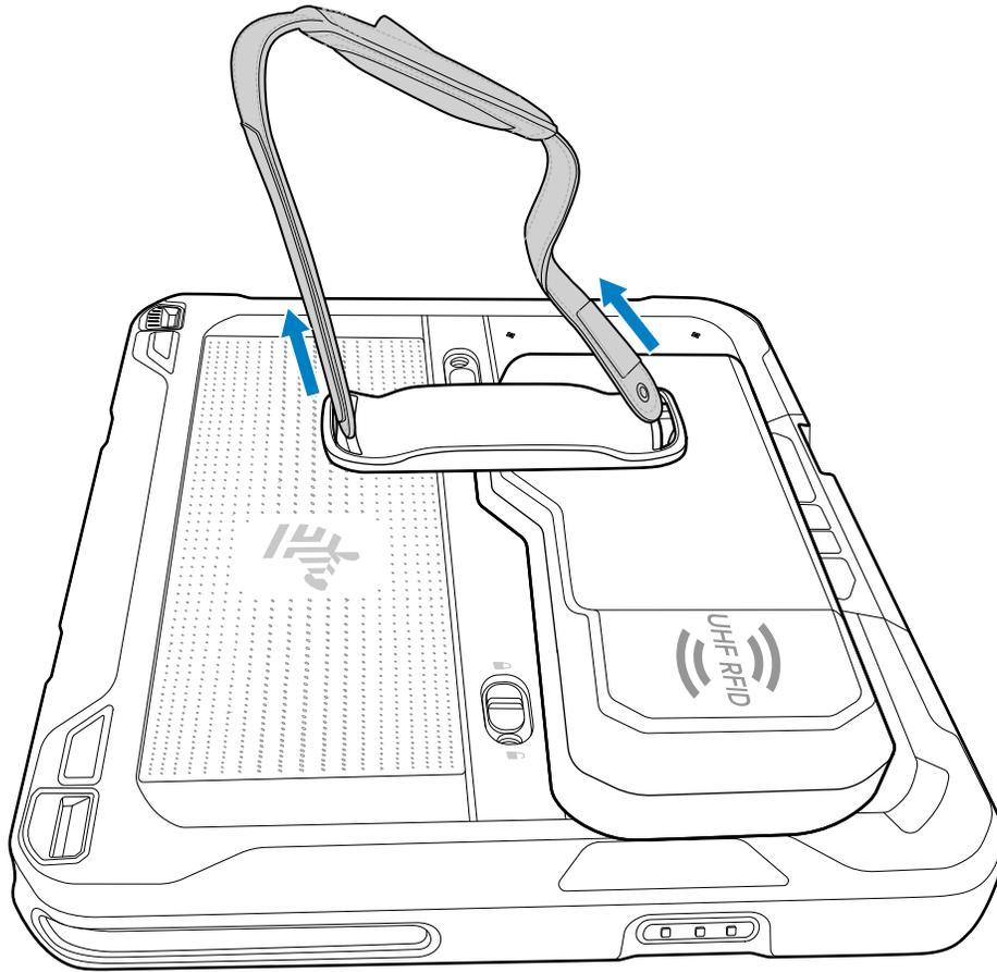
3. Insert the eyelet end of the replacement hand strap into the slot.
