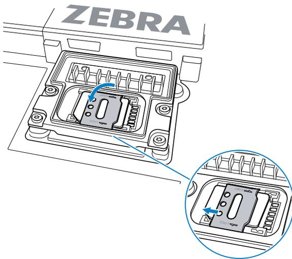
8. Slide the SIM holder to the lock position.
