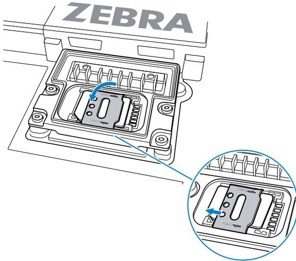
11. Slide the SIM holder to the lock position.
