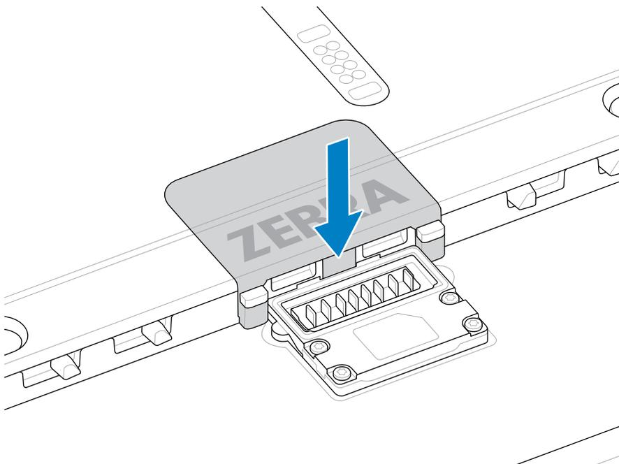
13. Insert the battery, bottom first, into the battery compartment at the back of the device.
