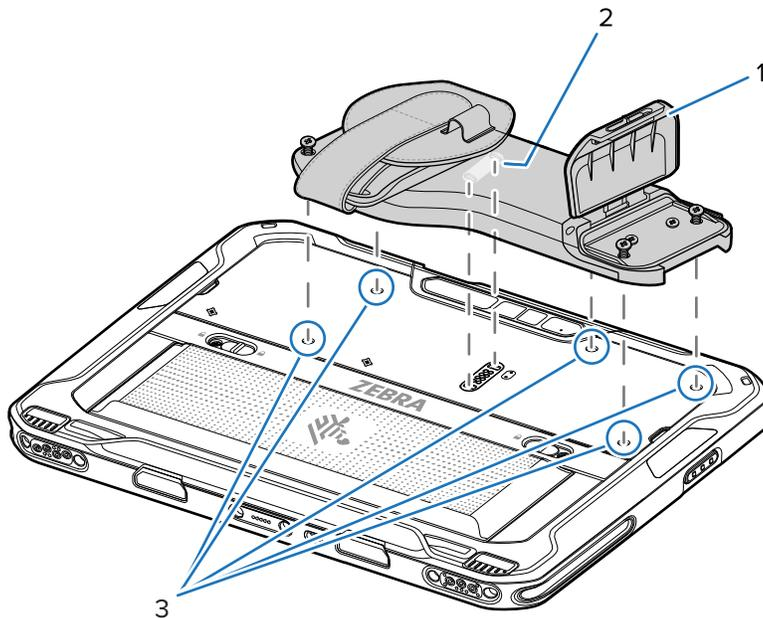
2. Align the two tabs (2) on the reader with the connector on the device.
