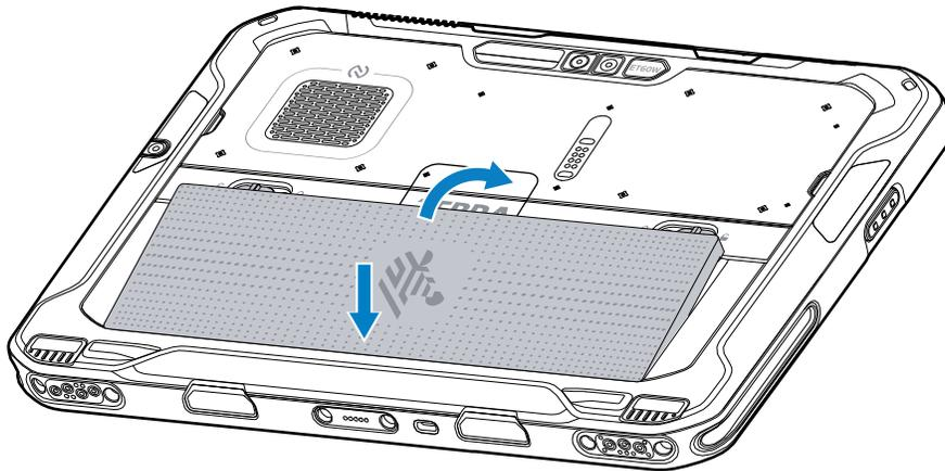
11. Press the battery down into the compartment until the release latches snap into place.
