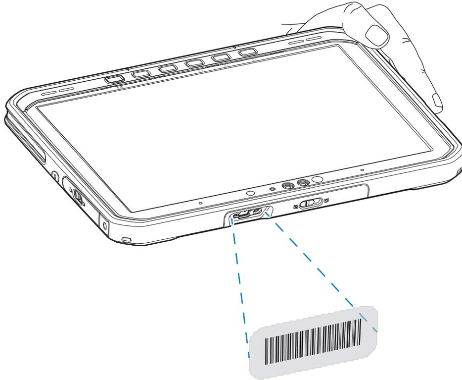
The aiming dot with illumination turns on to assist in aiming.
