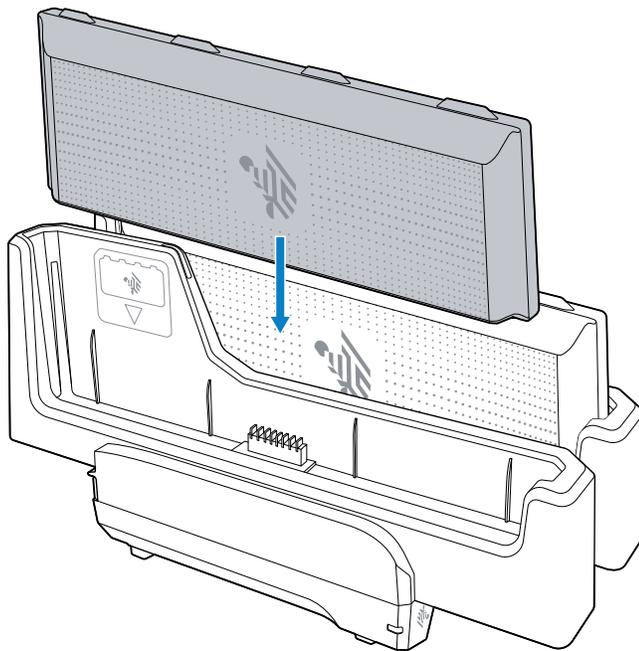
3. Gently press down on the battery to ensure proper contact.
