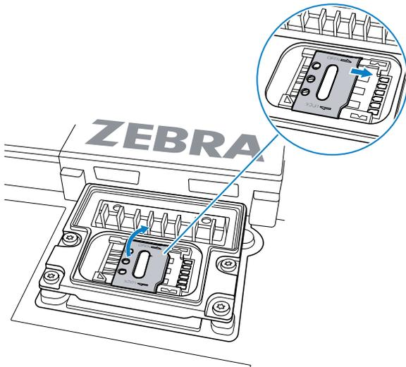
8. Lift the SIM card out of the SIM holder.
