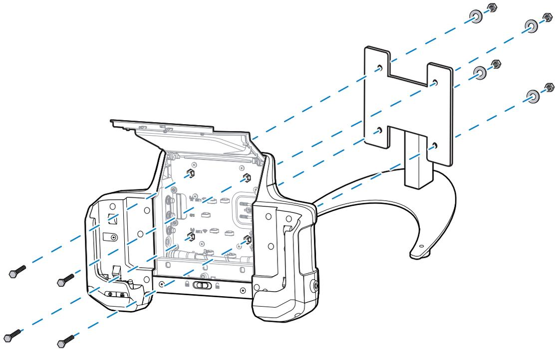
4. Insert the washers onto the bolts.
