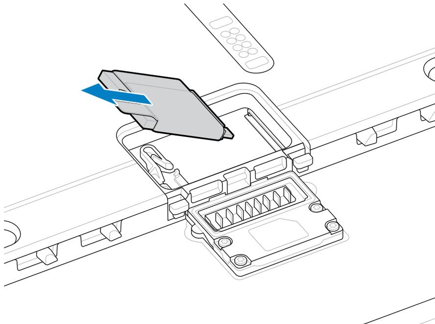
8. Align the replacement SSD with the connector on the board.
