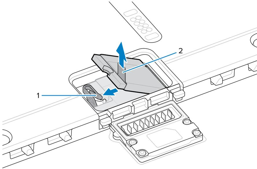
7. Remove the SSD from the connector on the board.
