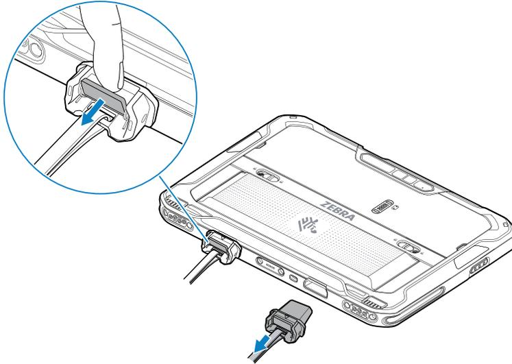
2. Pull the D-Clip out of the tablet.
