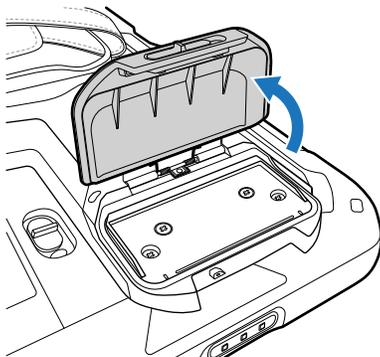
3. Insert the card (chip facing down) into the card slot (1).
