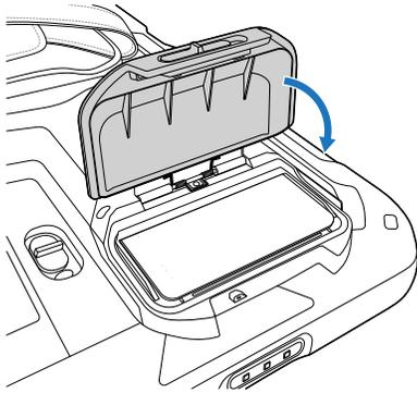
5. If required, secure the door with a M1.6 screw. Torque to 1.5 kgf-cm (1.3 lbf-in.).
