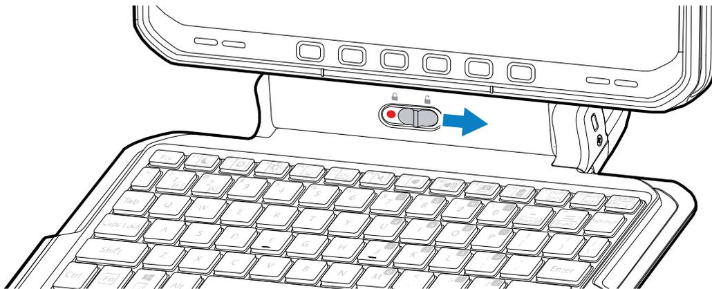
When in the unlock position, the orange indicator is visible to the left of the switch.
