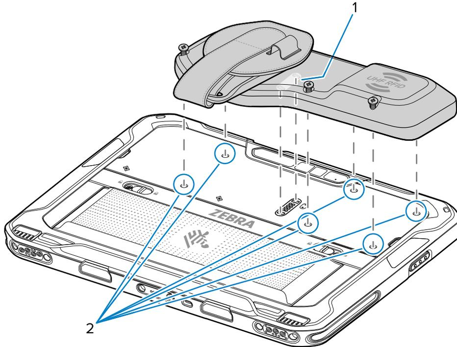
2. Press down on each screw to puncture the mylar (2).
