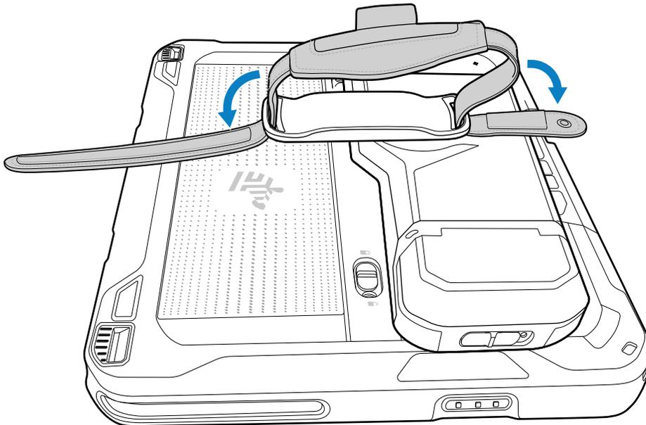
2. Pull both ends of the hand strap through the slots in the reader.
