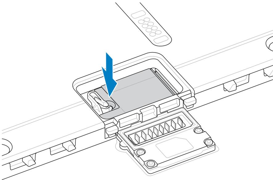
11. Align the SSD cover with the back of the tablet.
