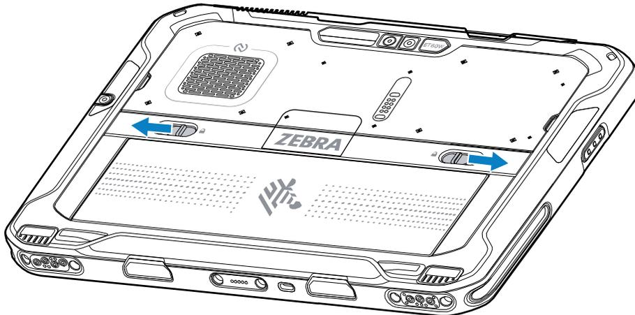
4. Lift the battery out of the tablet.
