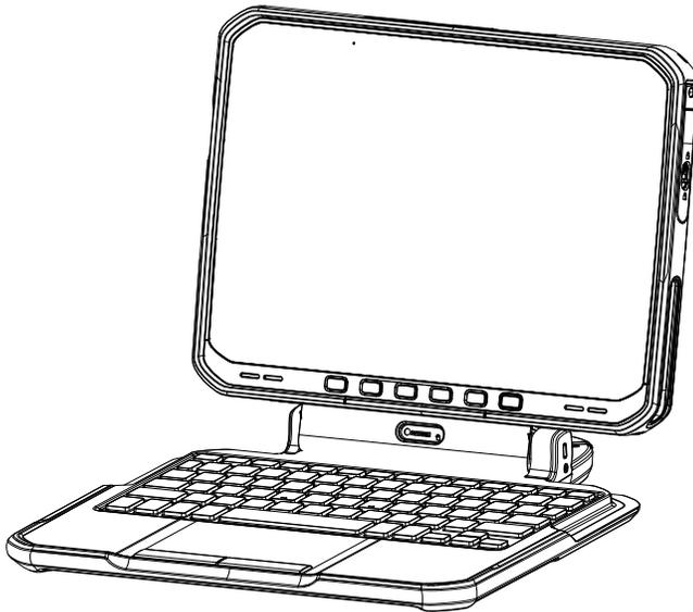
To close the keyboard, rotate the keyboard up.
