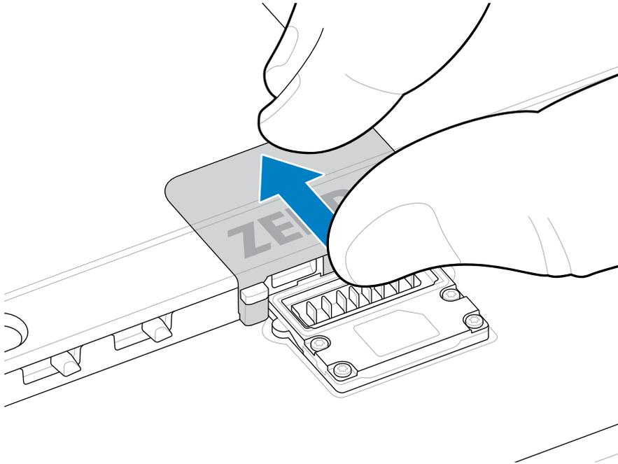
6. Push the locking tab (1) up and gently lift the SSD tab (2).
