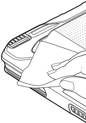
3. Align the Stylus Holder on to the tablet and press down to adhere to the tablet.
