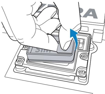
4. Slide the SIM holder to the unlock position.
