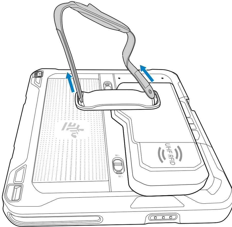
3. Insert the eyelet end of the replacement hand strap into the slot.
