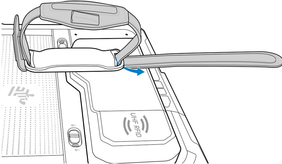
6. Fold the end up and press against the hook and loop material.
