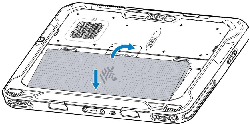
14. Press the battery down into the compartment until the release latches snap into place.
