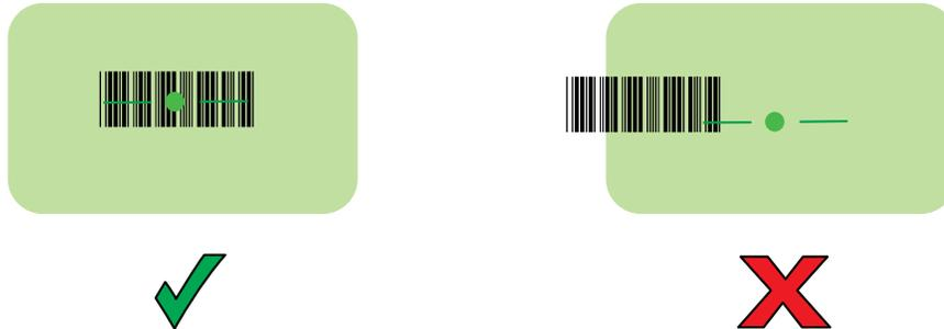
**Figure 13** SE55 Aiming for Pick List Mode with Multiple Barcodes
