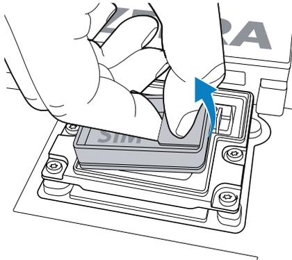
6. Slide the SIM holder to the unlock position.
