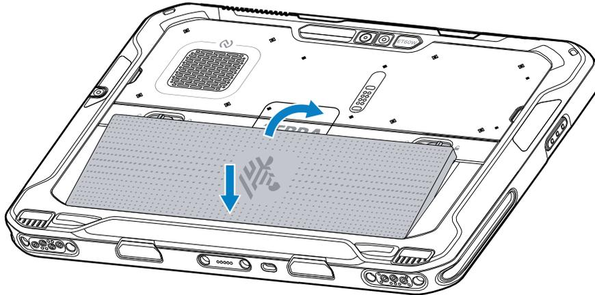
4. Press the battery down into the compartment until the release latches snap into place.
