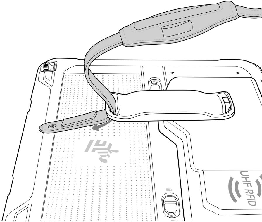
4. Fold the end up and press against the hook and loop material.
