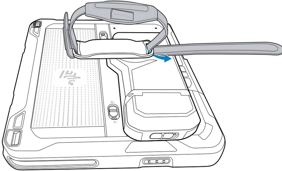
6. Fold the end up and press against the hook and loop material.
