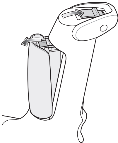
Figure 1-4 RFID Sled Battery Removal
