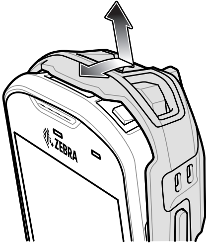
Figure 131 Lift Boot Over Device
