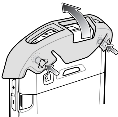
Figure 112 Rotate Top Cap Cover Top of Device
