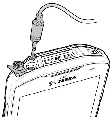
Figure 117 Audio Adapter Installation
