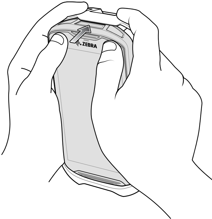
Figure 132 Push Device into Boot
