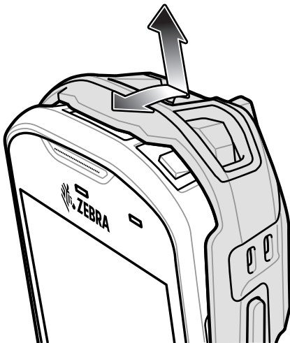
Figure 103 Lift Boot Over Device
