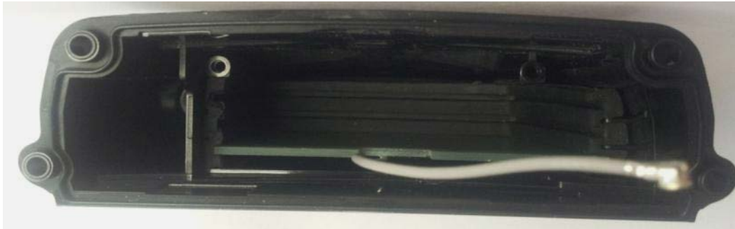
Figure 2-5 Antenna position for WLAN only WAP4 version
