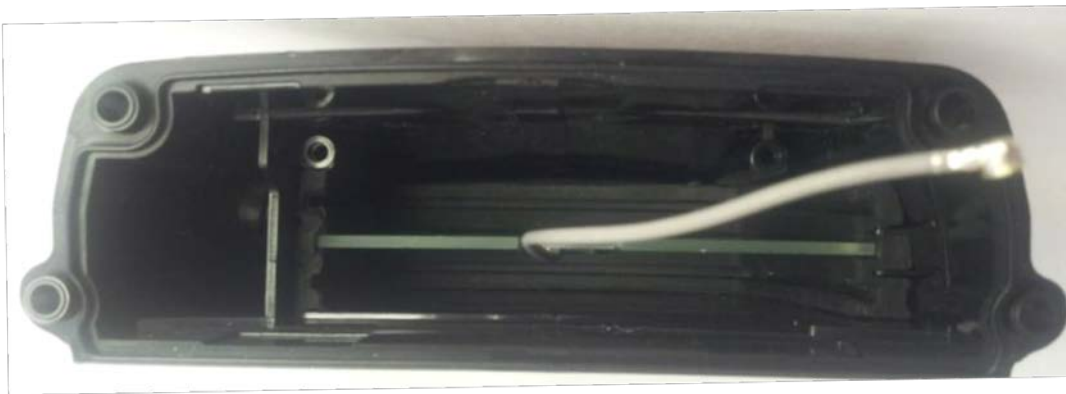
Figure 2-6 Antenna position for WWAN or GPS WAP4 version
