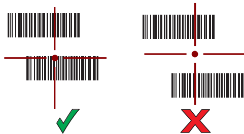
Figure 33 RS507/RS507X Pick List Mode with Multiple Barcodes in Aiming Pattern
