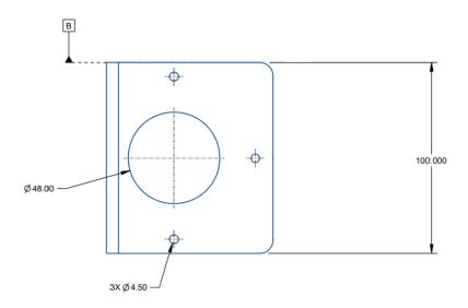
Figure 60 Light Bracket Dimensions
