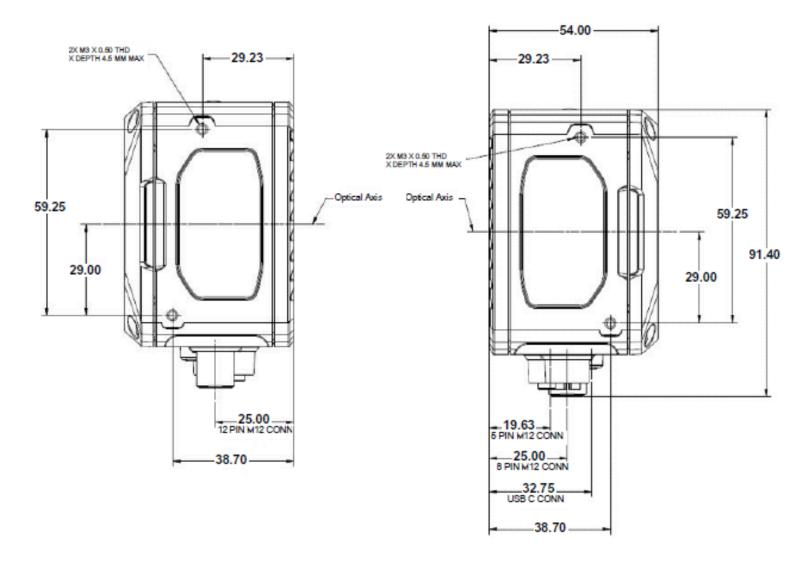
Figure 52 xS40 Front Mounting Holes
