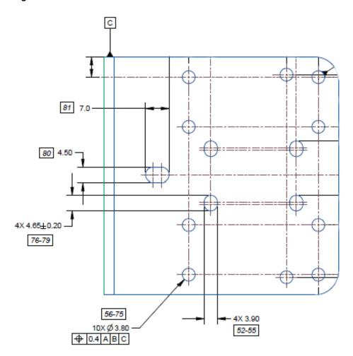
Figure 57 L Bracket Side Dimensions
