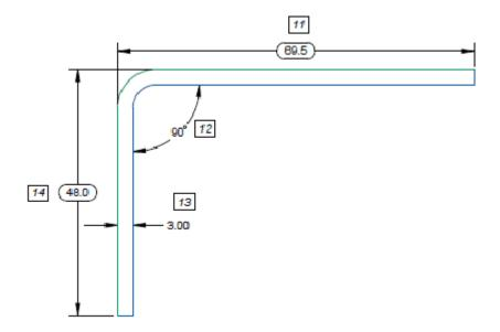
Figure 56 L Bracket Bottom Dimensions
