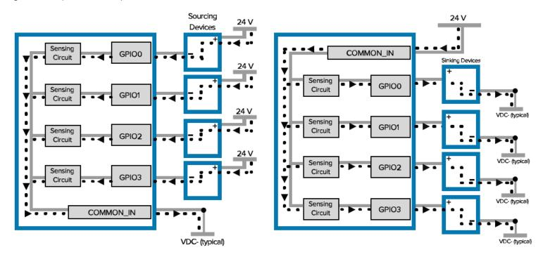
Figure 11 Opto-Isolated Outputs
