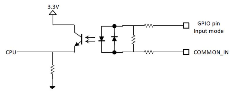
Optocoupled GPIO can operate non-isolated by terminating COMMON\_IN and COMMON\_OUT to the DC\_IN or GND wires that power the device.
