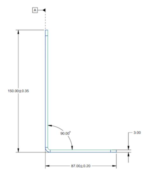
Figure 59 Light Bracket Dimensions
