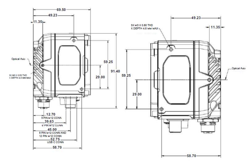
Figure 54 xS70 Front Mounting Holes
