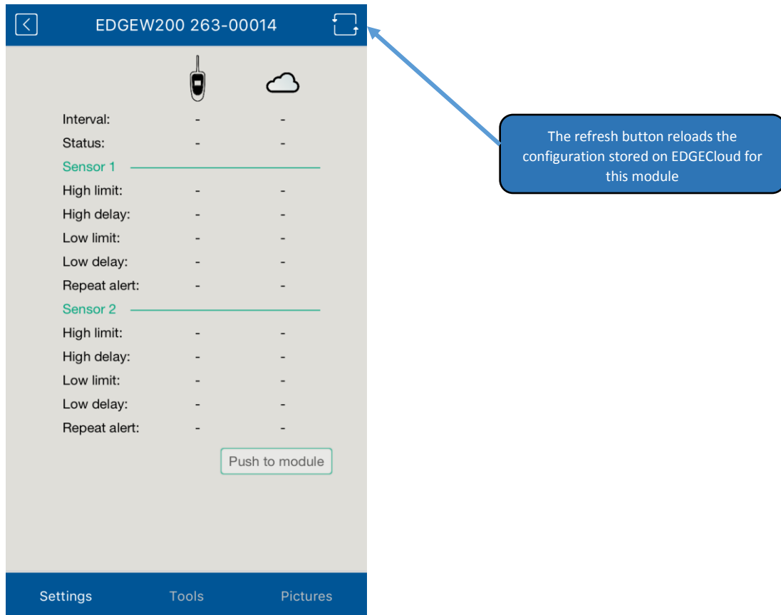
Figure 4 – No settings are shown until you make changes via the web application (EDGEConnect)
