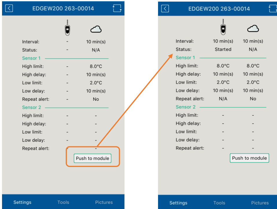
Figure 40 – Updating settings on EDGE sensor module with EDGEConnect Mobile application
