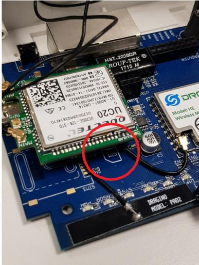
3. Insert your micro SIM card (contact facing up) in the SIM card slot.
