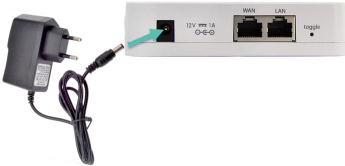
2. Plug the power adapter in to a wall outlet to turn on your gateway. When the device is ready for use, the green light turns on and remains on. The system LED blinks during OCEABridge startup.
