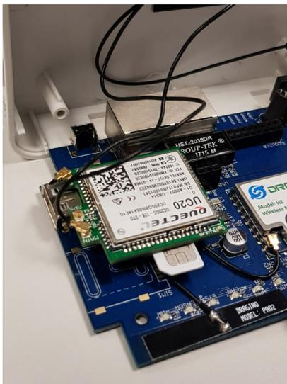
4. Insert the micro SIM card completely into the slot until it locks in.
