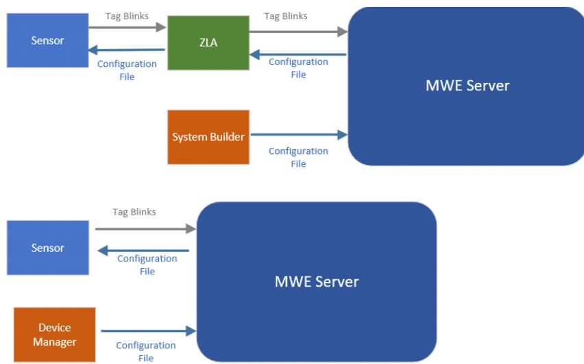
In the first case, a configuration file is created using the System Builder tool and published to a ZLA appliance, which publishes the file to the sensors. The sensors forward location data (tag blinks) to the ZLA and then to the MWE server.
