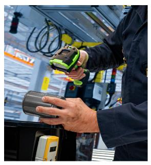
DS3600-DP and DS3600-DPA models bring the lightningfast capture of virtually every direct part mark to aerospace, automotive and other manufacturing plants where end-to-end traceability of product components is required.
