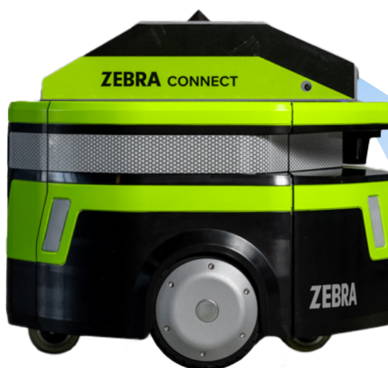
Floor-illuminating LED indicates motion and direction.
