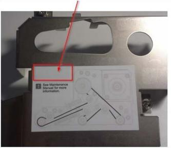
The presence of the extended life media drive system identification label indicates an extended life drive system is installed.
