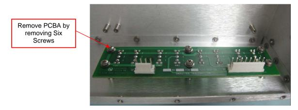
U) Disassemble the remaining sides and bottom from the Housing by unscrewing the remaining six Screws from each side and sixteen Screws from the Bottom Cover as follows:
