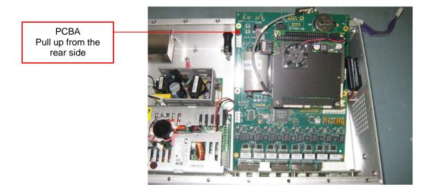
E) Remove two Cable Assemblies from the PCBA that was just removed:
