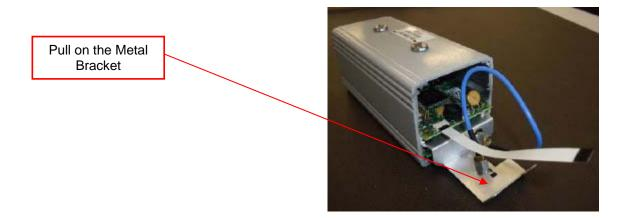
F) Remove two Cable Assemblies from the PCBA's. One Cable Assembly will be removed by unscrewing. The other is removed by placing a tool between the Cable Assembly and the Connector locking tab then pull on the connector to remove.
