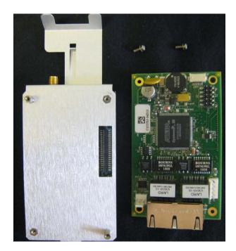
I) Turn the assembly over and remove the remaining PCBA from the metal bracket by unscrewing two screws:
