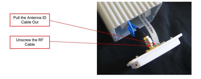
E) Pull remaining items from the housing by pulling on the Metal Bracket as follows:
