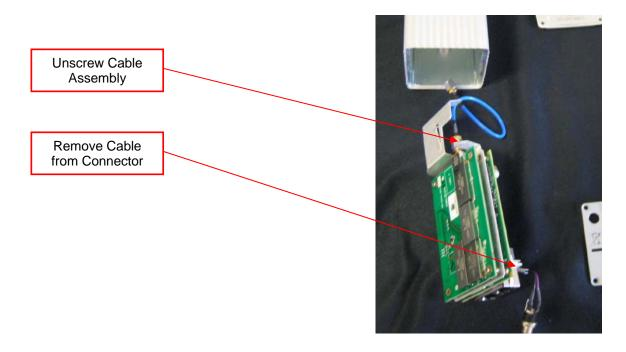
G) Remove the top Printed Circuit Boards (PCBA's) from the metal bracket by unscrewing two screws then pull the PCBA from the connector.
