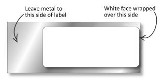
Smallest recommended bending diameter of the Confidex Silverline Blade II+™ is 100mm. For optimal performance please bend the label in the orientation shown below.
