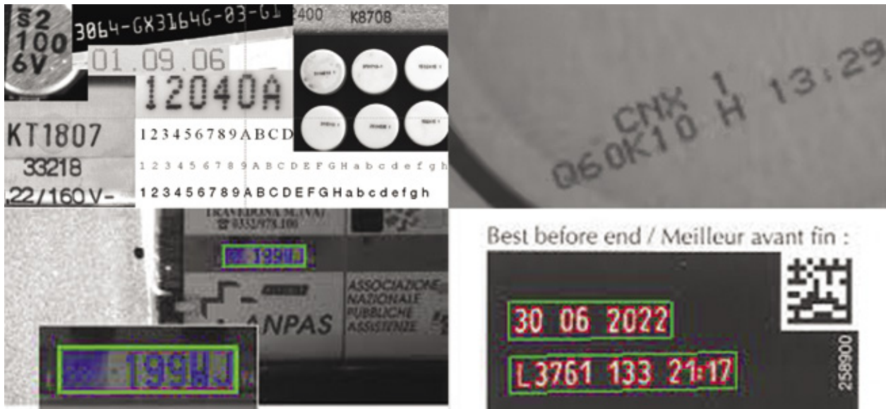
Figure 3: The OCR capabilities provided by the DL-OCR tool offer a solution for challenging character recognition projects. These projects involve complex backgrounds, blurry or damaged characters, distortion, or reflective surfaces that make traditional OCR techniques ineffective. The tool includes a pre-trained neural network, ready for use with thousands of diverse image samples. It achieves approximately 97% accuracy right from the start, even in very difficult scenarios.
