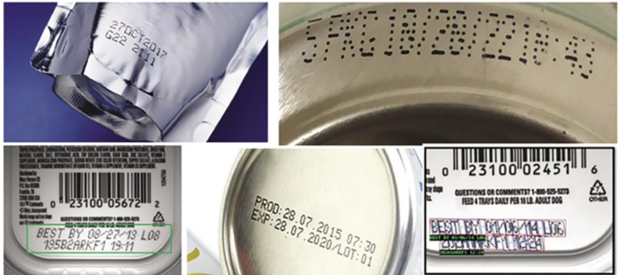
Figure 1: Traditional OCR methods may encounter challenges when dealing with reflective surfaces, printing on curved surfaces, and characters that are skewed, distorted, or obscured.
