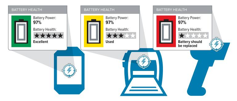
In other words, the health information available from Zebra's PowerPrecision batteries shows you when your battery is only operating at, for instance, 80 percent capacity (which is an indicator of a reduction in battery runtime).
