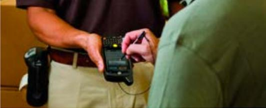
The **MC67** is an all-in-one device made for life in the field. It provides access to backend systems on the move, scans practically any barcode in any condition, captures whole documents in one snap, takes and sends video for real-time repair support, and functions as a phone so workers can call customers with an arrival window.
