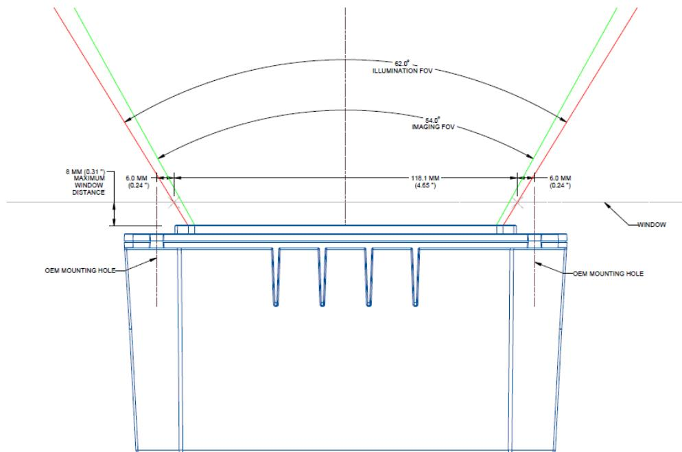
**Figure 5** SM72 Dimensions Side View
