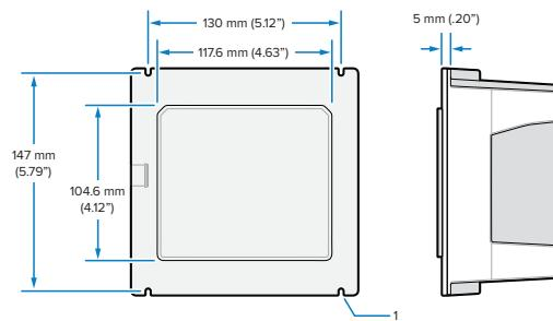
In the above figure, 1 shows the clearance slot for an M4 socket as used in [Panel Mounting with Threaded Studs](#).
