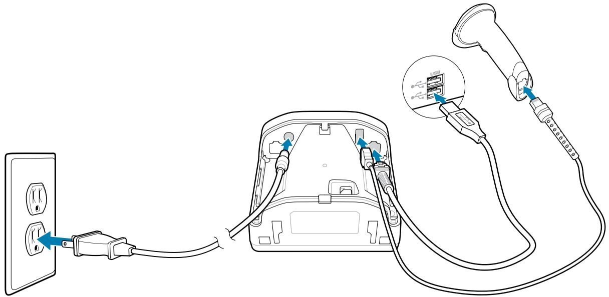
5. The scanner automatically detects the host and uses the default USB device type. If the default (\*) does not meet your requirements, select another USB device type by scanning the appropriate barcode from [USB Device Type](#).
