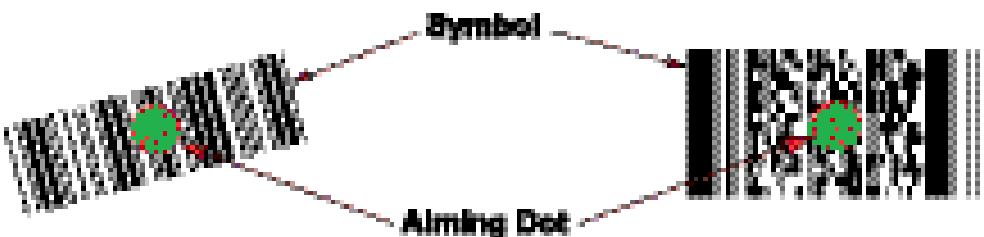
The digital scanner can also read a barcode presented within the aiming dot not centered. The top examples in [Figure 20 on page 48](#) show acceptable aiming options, while the bottom examples can not be decoded.
