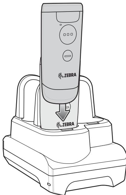
The CS6080 begins charging. The charge status LEDs light to indicate progress. See [Beeper and LED Indications on page 39](#) for more information.
