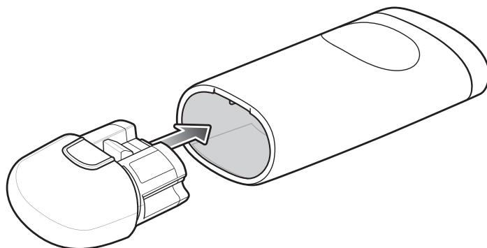
2. Press the battery into the scanner until the battery snaps into place.
