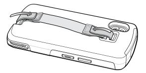
**4.** Place hand between device and hand strap and adjust hand strap as necessary.
