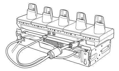
**11.** Secure top tray to bottom tray with four M5 screws (two on each side).
