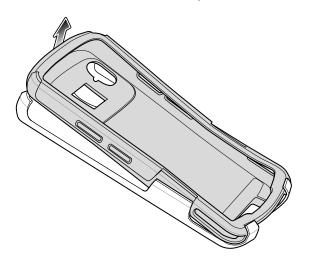
**2.** Insert the bottom of the device into the bottom of the boot.
