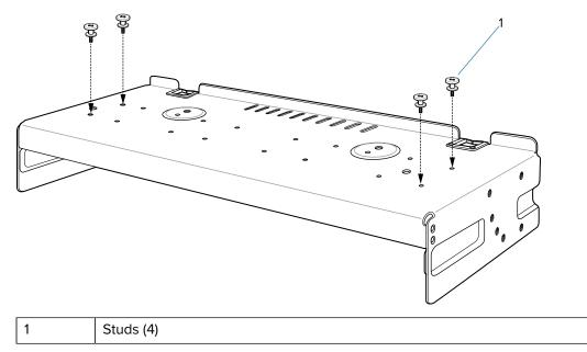
7. Align and install 5-Slot cradle onto studs of top tray.
