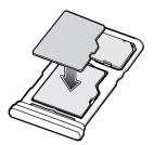
**4.** Insert the SD/SIM card drawer into the device.
