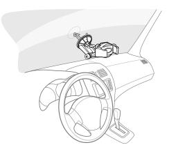
2. Push the lever towards the base to create a vacuum between the suction cup and the windshield.
