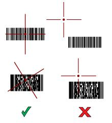
Figure 12 RS507/RS507X Aiming Pattern
