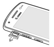
**3.** Insert or replace the microSD card into the SD/SIM card drawer.
