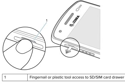
**2.** Remove the SD/SIM card drawer from the device.
