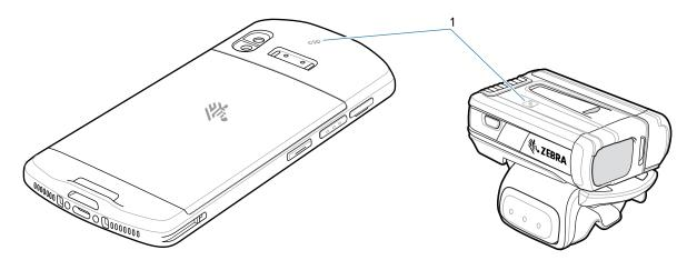
The Status LED blinks blue indicating that the Ring Scanner is attempting to establish a connection with the device. When a connection is established, the Status LED turns off and the Ring Scanner emits a single string of low/high beeps.
