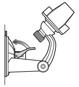
**3.** Make sure that the suction bond is strong enough before installing the device.
