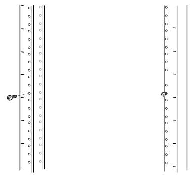
**3.** Align the mounting bracket's top mounting key holes with the screws.
