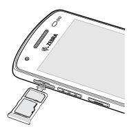
5. Press the SD/SIM card drawer into the device to ensure it is in securely.
