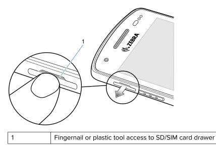
**2.** Remove the SD/SIM card drawer from the device.
