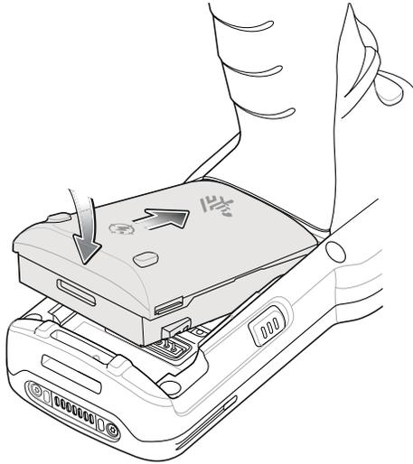
3. Slide the front of the battery into the battery compartment.
