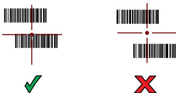
Figure 13 RS6000 Pick List Mode with Multiple Barcodes in Aiming Pattern
