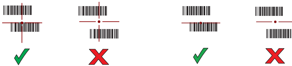
Figure 5 Pick List Mode with Multiple Barcodes in Aiming Pattern: Standard and Extended Range
