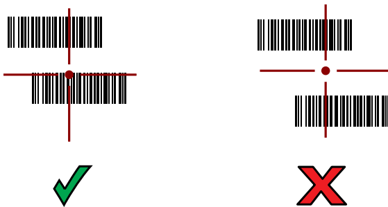
Figure 16 RS507/RS507X Pick List Mode with Multiple Barcodes in Aiming Pattern
