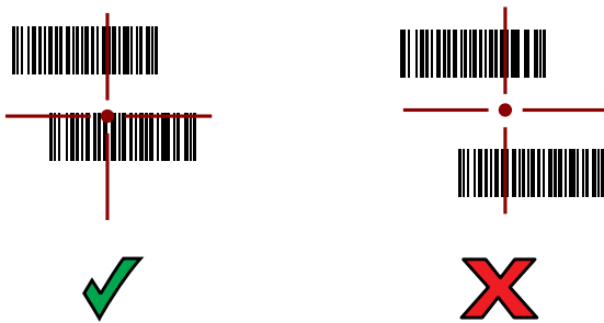
Figure 10 RS5100 Pick List Mode with Multiple Barcodes in Aiming Pattern
