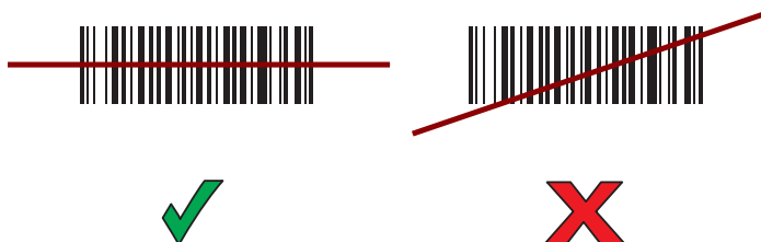
Figure 7 Linear Scanner Aiming Pattern
