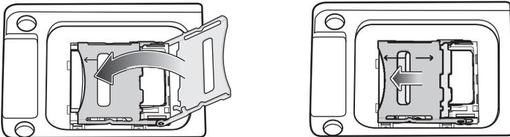
6. Replace the microSD card cover and ensure that it is installed properly.
