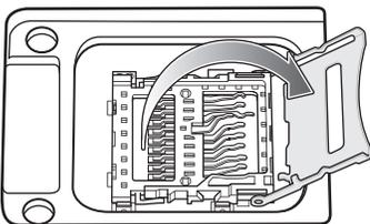
4. Place the microSD card into the contact area with the contacts facing down.
