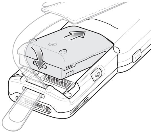
3. Slide the front of the battery into the battery compartment.
