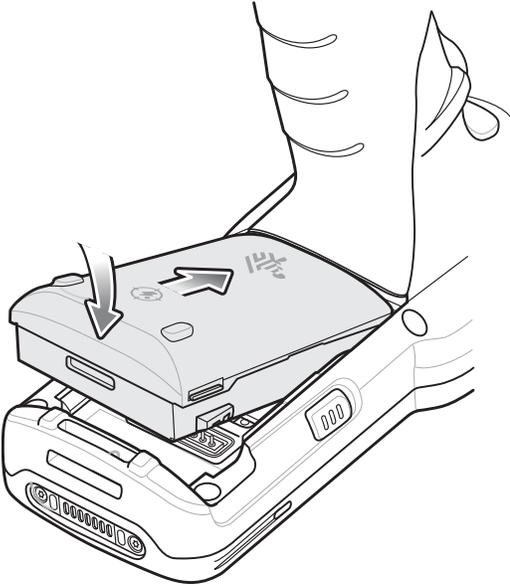
4. Slide the front of the battery into the battery compartment.
