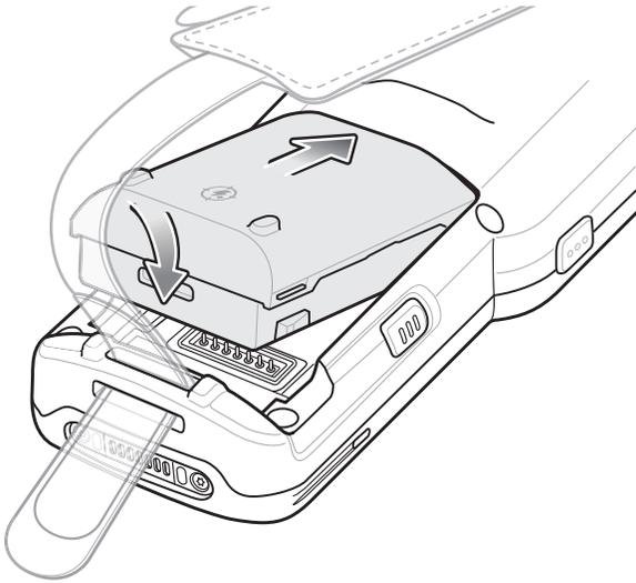
4. Slide the front of the battery into the battery compartment.
