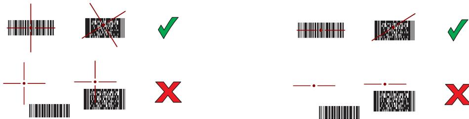
**Figure 39** Pick List Mode with Multiple Barcodes in Aiming Pattern: Standard and Extended Range
