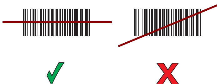
Figure 11 Linear Scanner Aiming Pattern
