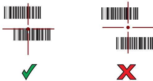
Figure 14 RS507/RS507X Pick List Mode with Multiple Barcodes in Aiming Pattern
