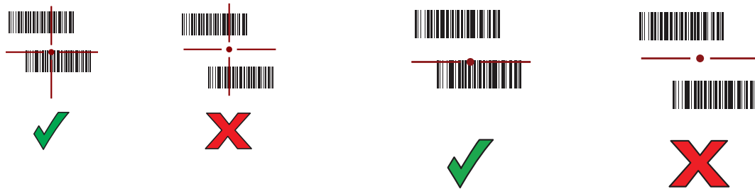
Figure 9 Pick List Mode with Multiple Barcodes in Aiming Pattern: Standard and Extended Range
