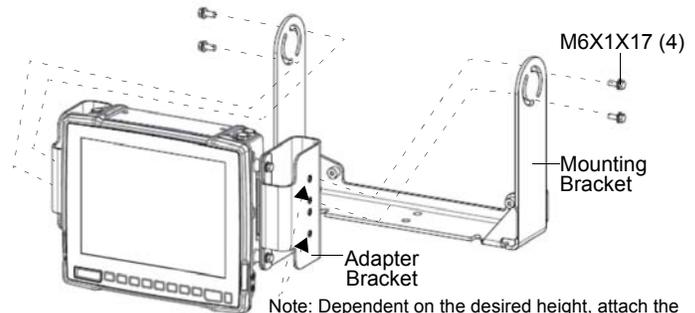
Note: Dependent on the desired height, attach the U-Mount Bracket to either the top two or bottom two holes located on the Adapter Bracket.
