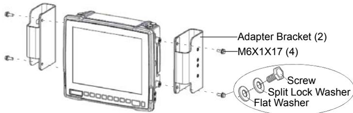
2. Mount the Mounting Bracket (P/N: VM1010BRKT) in the desired location using the M10X1.5X50 screws, split lock washers, and flat washers (not included in the Adapter Bracket kit). Torque the screws to 42 Nm (31 ft-lbs).
