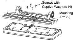
2. Attach the left and right mounting arms to both sides of the VC70, using the M5x14mm Torx head screws with flat and lock washers. Only tighten the cap screws three turns.
