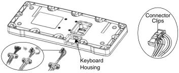
2. Turn the connector on the cable straight (with connector clips on top) and plug the connector in the keyboard.
