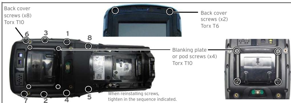
5. Carefully separate the back cover from the main housing. Disconnect any connecting wires.
