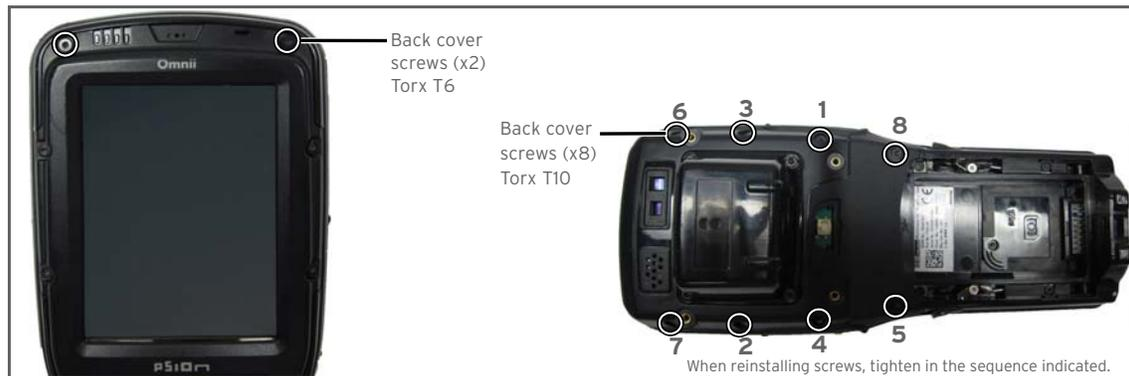
3. Gently pull the back cover away from the main housing, being careful to not put stress on any cables connecting the two parts.
