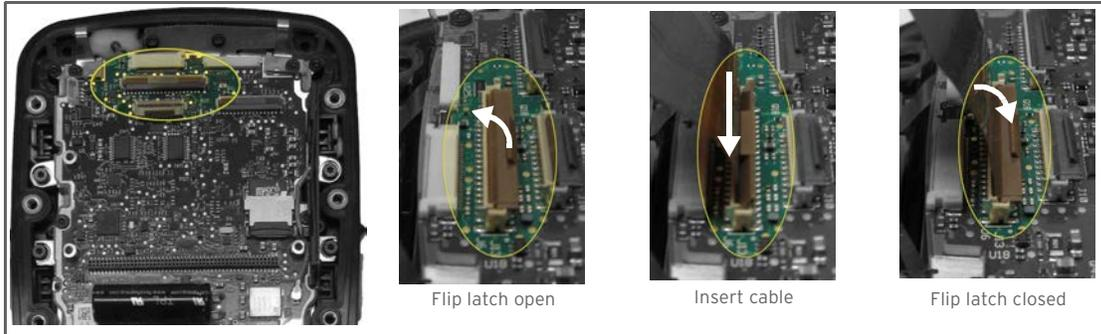
4. Insert the pistol grip trigger wire harness in the white socket on the left side of the main logic board.
