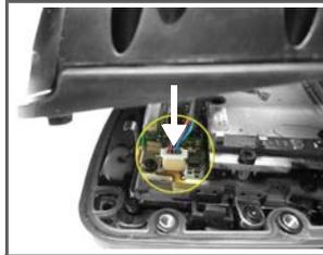
5. Fit the back cover in place against the main housing, ensuring that no cables are caught in the seal.
