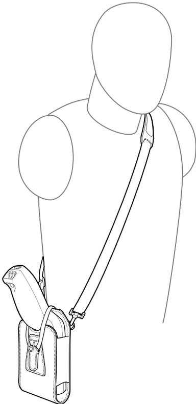
3. Lift the strap and insert the device into the soft holster, with the screen facing the user.
