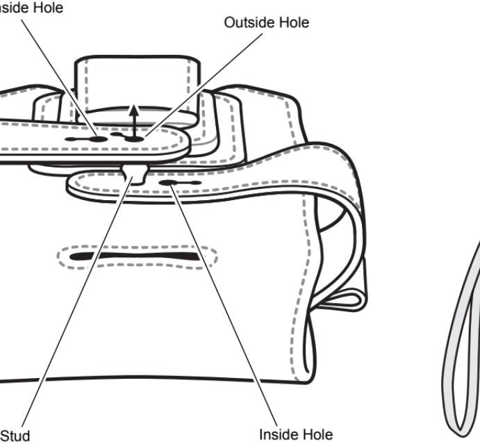
Insert the Trigger Handle, with display facing in and the scanner facing down into the holster.
