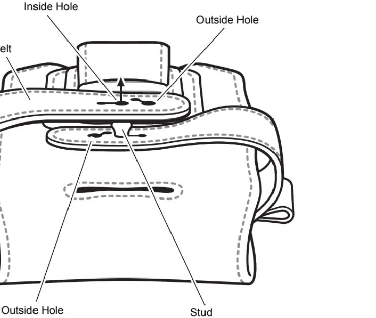
Insert the device, with display facing in and the scanner facing up into the holster.
