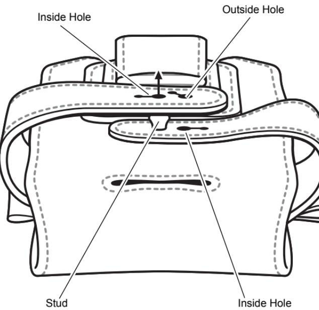
Insert the device with Rugged Boot, with display facing in and the scanner facing up into the holster.
