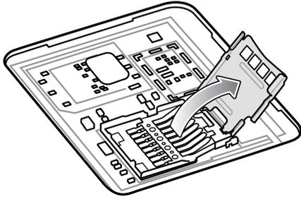
4. Insert the microSD card into the card holder door ensuring that the card slides into the holding tabs on each side of the door.
