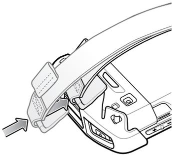
7. Push the clip onto the top cap.
