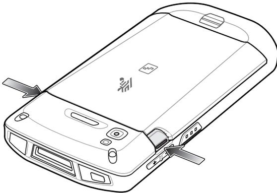
7. Lift the battery from the device.
