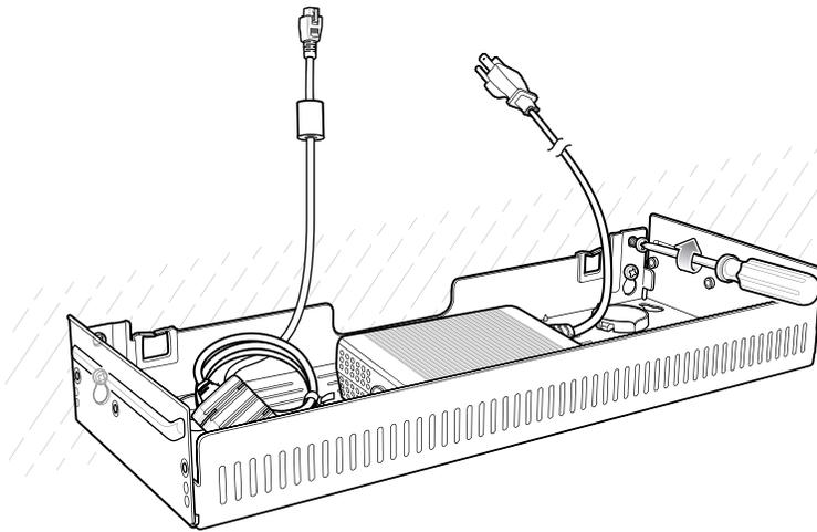
7. Assemble the four 4-Slot Battery Chargers or cradle onto the bracket. See steps 7 through 11 on [page 157](#).
