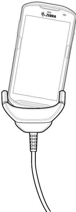
2. Rotate the device into the cup.
