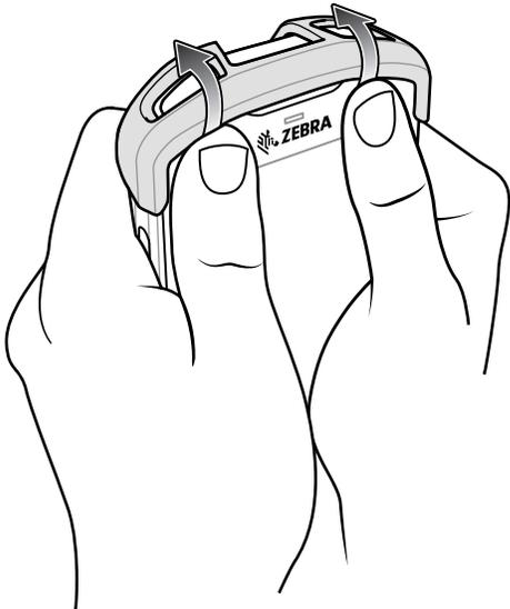
2. Pull the strap tab through the cut slot.
