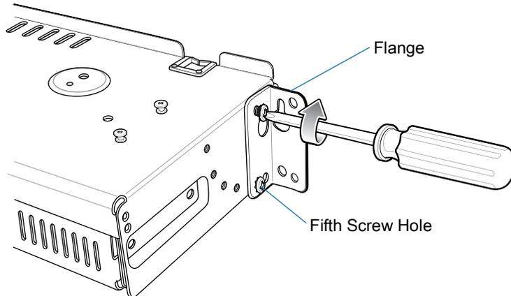
**Figure 70** Flange 25° Position (4-Slot Battery Chargers)
