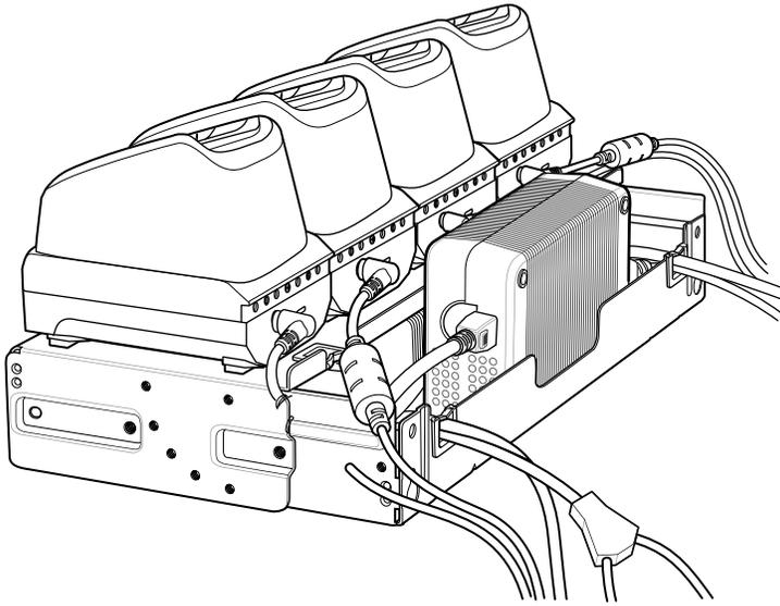
11. Secure top tray to bottom tray with four M5 screws (two on each side).
