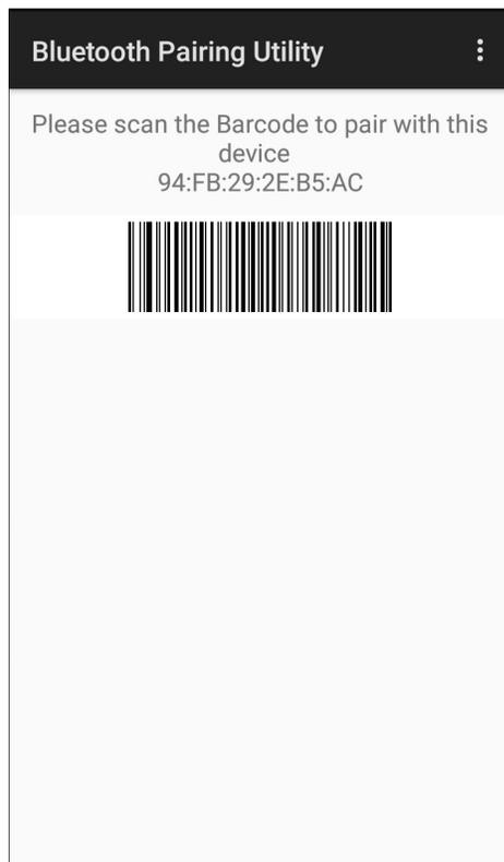
4. Using the scanner, scan the barcode on the screen.
