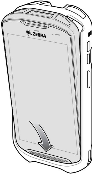
2. Lift the top of the Rugged Boot over the top of the device.
