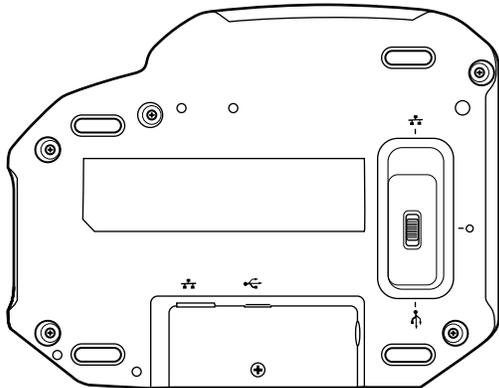
For Ethernet communication, slide the switch to the
