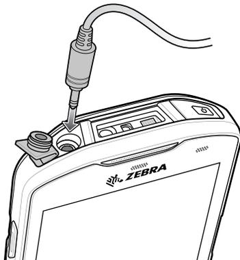
3. Connect the 3.5 mm connector plug of the headset into the 3.5 mm Audio Adapter.
