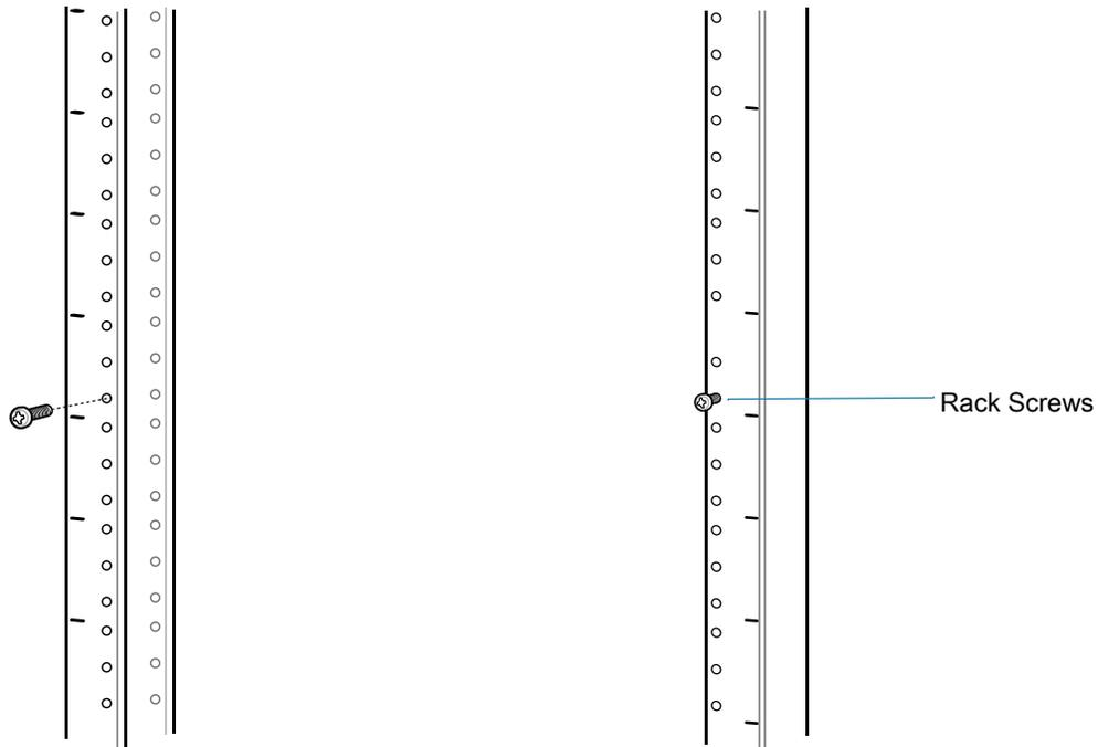
3. Align the mounting bracket's top mounting key holes with the screws.
