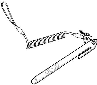
4. Insert the loop into the hand strap holder.
