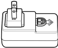
2. Rotate the plug adapter up and out of the power supply.
