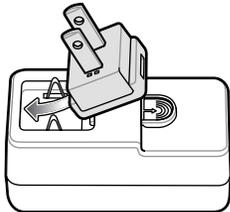
4. Rotate the plug adapter down and snap into place.
