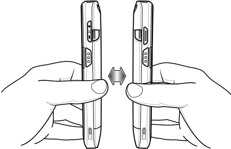
When the devices connect, a sound emits, the image on the screen reduces in size, the message **Touch to beam** displays.
