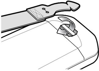
5. Feed the tab into the cut in the strap.
