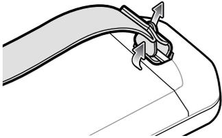
6. Align the hand strap clip with the top cap.
