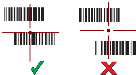
Figure 18 RS507/RS507X Pick List Mode with Multiple Barcodes in Aiming Pattern
