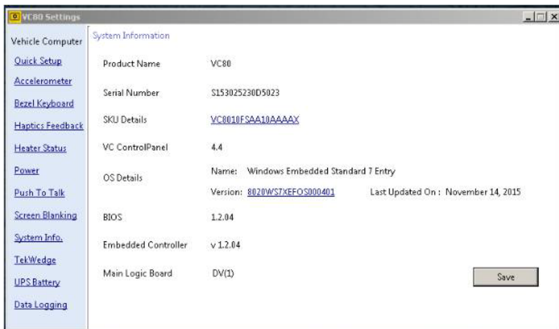
Figure 3-23 System Information (VC80 with Windows 7)
