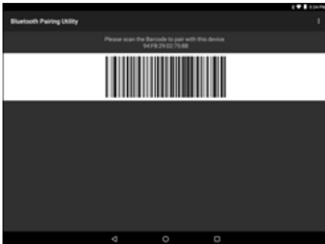
4. Using the scanner, scan the barcode on the screen or scan the barcode on the right side of the VC80x.
