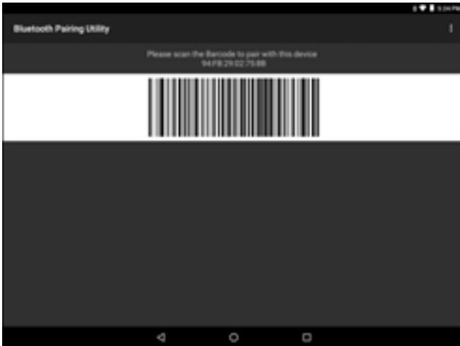
4. Using the RS507/RS507x/RS6000, scan the barcode on the screen or scan the barcode on the right side of the VC80x.
