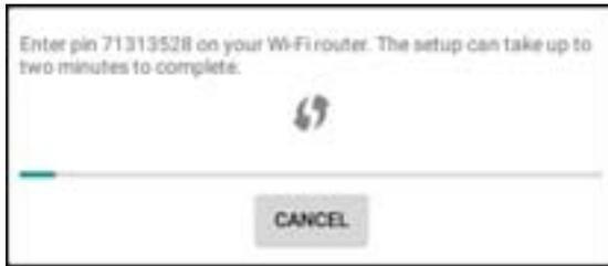
5. On the router, enter the Pin number. The VC80x connects to the wireless router.
