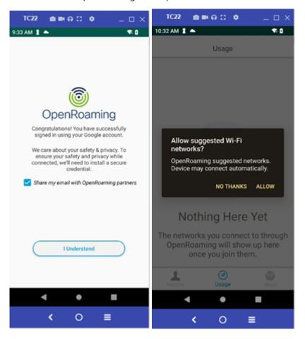
**8.** If not using a cellular connection, go to Wi-Fi settings. The Zebra device auto-connects to the **OpenRoaming** SSID in the Wi-Fi scan list when you disconnect from the current WLAN profile.
