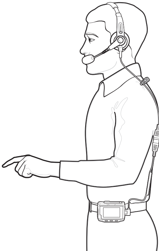
Figure 6-31 Long Quick Disconnect Audio Cable Connection to Headset
