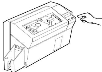
3. A test card will print after a few seconds. LCD display will show printing status. Test Card is printed on both sides of the card.
