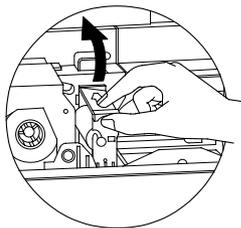
3. Make sure the arrow on top of the assembly is facing toward the rear of the printer. Hook assembly into slot on printer and rotate down. Ensure the assembly locks in place.
