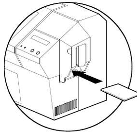
A Manual Feed Slot is available on the side of the Card Feeder cover for feeding single cards. Cleaning Cards are fed manually through this slot.
