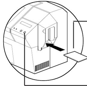
**2.** Insert one Pre-Saturated Cleaning Card (provided) through slot on the side of the Card Cartridge.
