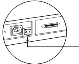
2. Place the printer's power switch in the OFF (0) position.
