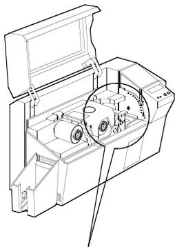
2. Open Printer cover and remove the yellow reminder tape from the location for the Cleaning Cartridge.
