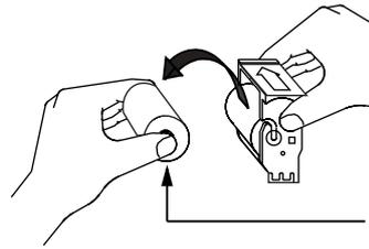
3. Remove Cleaning Roller from Cartridge and discard.
