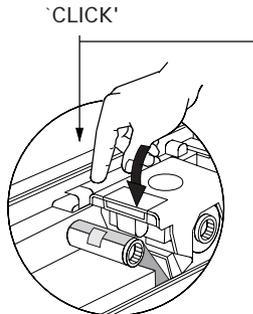
4. Push down on the Print Head Lock Lever until an audible 'click' signals the locked-down position.
