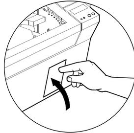
**3.** Swing the Rejected Card Box Door and press the top. An audible "click" signals the locked position.
