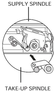
3. Load ribbon onto the supply spindle (under print head carriage) and empty core (with tape attached) onto the take-up spindle. Make sure the ribbon comes off of the top of the supply spindle and feeds to the top of the take-up spindle.
