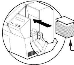
2. Install cards into Feeder\* as shown.
