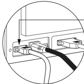
When a command to the parallel printer interface sends a card to the Smart Card Contact Station, the printer connects the Smart Card Contact Station to the female DB-9 connector on the rear of the printer.
