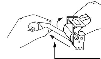
5. Carefully peel off wrapper from new Cleaning Roller while in Cartridge.
