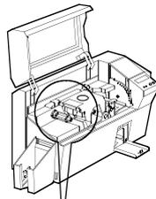
2· With printer power ON and READY status, open cover and press down on the Print Head Unlock Lever to open the print head carriage. The print head carriage will pop open.
