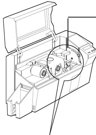
*2. Gently remove Cleaning Cartridge by rotating up and away from printer.*
