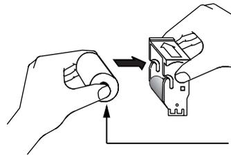
4. Install new Cleaning Roller into Cartridge\*. To avoid contamination, always hold the Cleaning Roller assembly by the ends.
