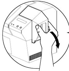
1. Open Card Feeder Cover by putting your fingers on both sides and rotating the cover in a clockwise direction to the open position.
