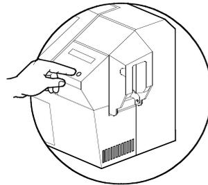
1. When the printer displays **READY**, press the “Next” button (left) on your Control Panel to “**SELF TEST CARD MENU**”, then the “Select” button (right).
