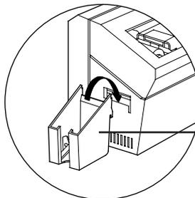
Install Card Output Hopper onto printer by hooking over bottom edge of card exit aperture.
